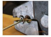
3. If not done so previously, the ferrule should then be placed inside the relevant size opening within the jaws
