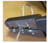
2. The size of the eye should be determined and prior to pressing a 'tail' of 2 x rope diameter should protrude from the end of the ferrule
